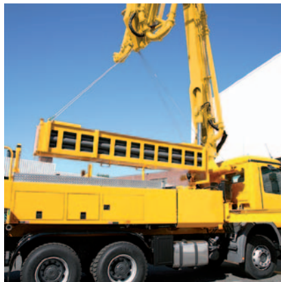
Additional storage boxes for hoses and pipes can be loaded and unloaded by fork lift, crane or the pumps own boom to place them where they are needed.
