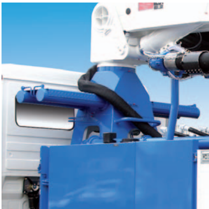
2 slewing cylinders on each side of the turret guarantee safe and dependable operation.
